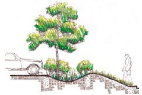
Parking Lot Island Bioswales
